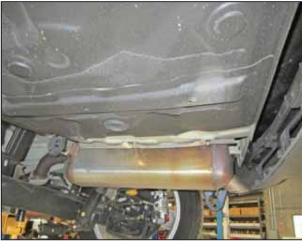
a. Stock exhaust system installed.
