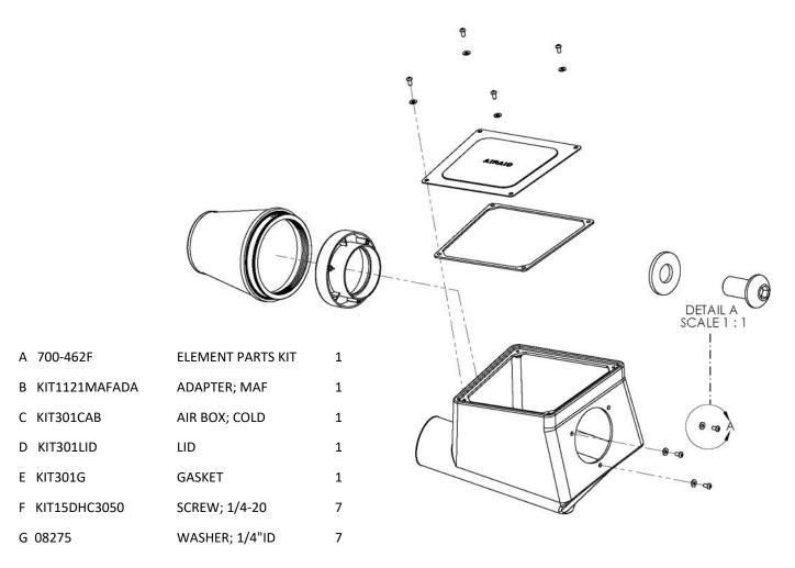
Create the U.B.I. Air Box assembly using the exploded view as a guide. Mounting holes can be drilled in any location as needed. 3/8" or 8mm hardware with flat washers is recommended but not required.
