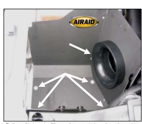
7. Install the air filter adapter (#4) using three  $^{1}4$ - $^{2}0x$   $^{1}2$ " button head bolts (#12), and  $^{1}4$ " flat washers (#13). Position the Airaid Cool Air Dam in place of the factory airbox & secure it with four M6-1x25 hex bolts (#14) and  $^{1}4$ " flat washers (#13).
