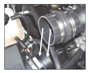
**10.** Install the urethane hump hose (#6) onto the Airaid Intake Tube (#5) and the MAF sensor with two #60 hose clamps (#15). Install the tube assembly onto the engine. (Hint: slide the hump hose all the way onto the end of the
