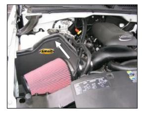
12. Press the weather strip (#8) along the top edges of the Airaid Cool Air Dam; assure that it is fully seated along the edges. (Hint: Begin at a corner and work toward the ends). Mount the Airaid Premium Filter (#1) onto the air filter adapter and tighten the hose clamp. Apply the Airaid decal inside the Airbox as shown.
