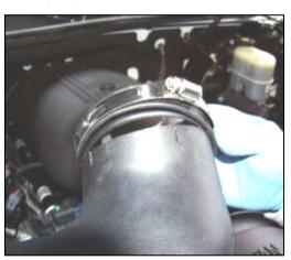
**9.** Install the GM coupler (#7) onto the throttle body side of the Airaid Intake Tube (#5).
