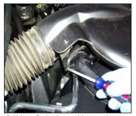
**3.** Using a flat head screwdriver, gently pry the radiator hose bracket from the factory intake tube assembly and remove the intake tube from the vehicle.
