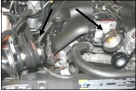
11. Install the urethane hump hose (#6) on the Mass Air Flow sensor with two #60 hose clamps (#15). Next install the urethane coupler (#7) on the throttle body with two #64 hose clamps (#16).
