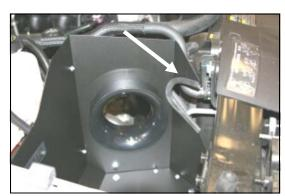
**9.** Install the assembled **CAD** in place of the factory airbox using four bolts (#11) and washers (#10). Do not over tighten the bolts. Install the rubber trim (#17) as shown at the arrow.
