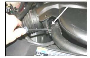
**3.** Using a screwdriver, pry the factory tube away from the plastic clamp on the radiator hose, and remove the tube.
