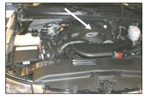
1. <u>Disconnect the negative battery cable.</u> Using a 5/16" socket, remove one bolt on the top of the beauty cover. Set the bolt and the cover aside for re-installation later.
