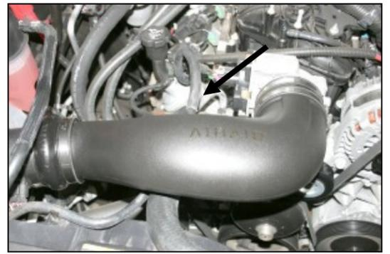
12. Install the Airaid Intake Tube into the hump hose first, and then onto the throttle body. Adjust it for fit, and tighten the hose clamps. Next install the 3/8" x 14" breather hose (#8) between the 1/4" NPT x 3/8" barbed fitting in the tube, and the factory port on the valve cover.
