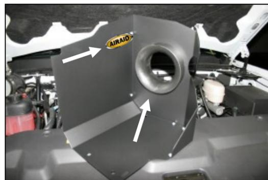
8. Assemble the **Cool Air Dam panels (CAD)** (#2 & #3) using five 6-32 x 5/16" screws (#10), #6 flat washers (#11), and 6-32 keps nuts (#12). Next install the air filter adapter (#5) into the panels as shown with the hole for the **Mass Air Flow** sensor facing up, using three 1/4 - 20 x 1/2" button head bolts (#14), and 1/4" flat washers (#15). Place the Airaid Decal on the panel as shown.
