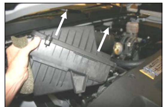
6. Rock the factory airbox back and forth to loosen it from the mounting grommets, and remove it from the vehicle.
