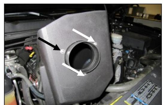
**9.** Install the Filter Adapter (#4) onto the Cold Air Box, or CAB (#3), as shown using the three 1/4-20 Button Head Bolts (#9) and 1/4" Washers (#10).
