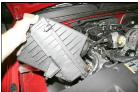
**7.** Rock the factory airbox back and forth to loosen it from the mounting grommets, and remove it from the vehicle.
