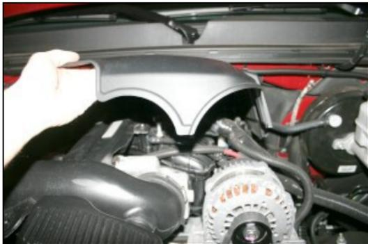
**1. Disconnect the negative battery cable.** Remove the factory engine cover by lifting up on the front, and then pulling the cover towards the front of the vehicle. It is only held in place with grommets.
