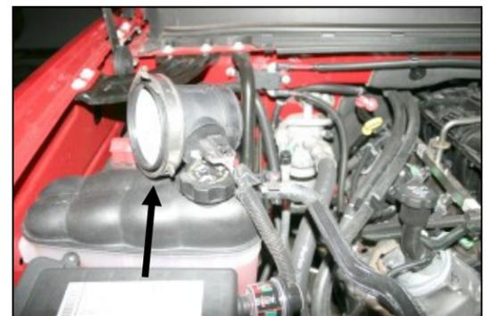
**6.** Remove, and set aside the MAF sensor from the factory airbox using caution to retain the factory clamp and seal.
