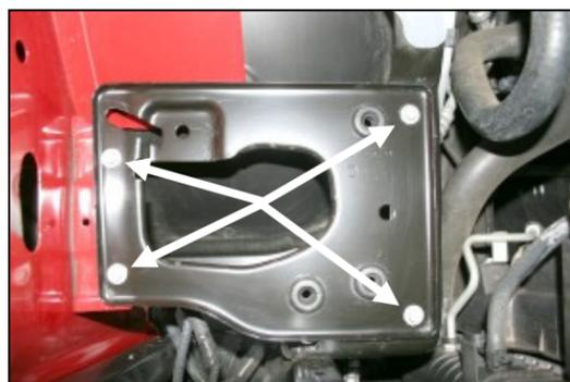
**8.** Using a 10mm socket, remove four bolts, and then remove the factory airbox mounting plate from the vehicle and set aside. Three of these bolts will be reused in step 11.
