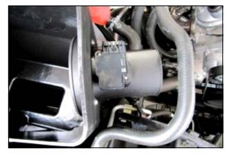
**10.** Transfer the Mass Air Flow sensor from the factory airbox into the Filter Adapter. Secure the sensor using the two 8-32 Button Head Screws (#9).
