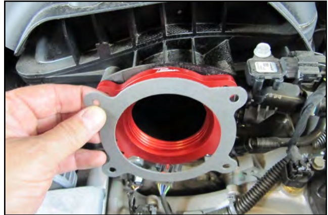
3. Install the AIRAID Spacer into the intake manifold with the supplied gasket on the throttle body side, as shown. *Note: AIRAID spacer must be installed with bore protruding into intake manifold away from throttle body. Incorrect installation will hinder performance. Reference picture below for spacer orientation
