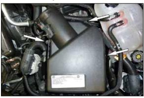
Loosen the three screws that secure the air filter housing lid and then lift up the housing and set
