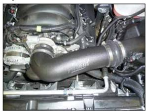
9. Install the AIRAID® intake tube into the hump coupler and then the coupler at the throttle body, adjust the tube for best fit and secure with the provided hose clamps.
