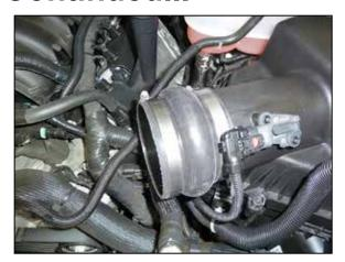
7. Install the provided hump coupler onto the filter housing and secure with the provided hose clamp.
