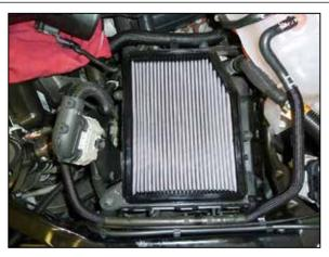
5. Remove the factory air filter and replace with the AIRAID® air filter provided. Reinstall the air filter housing lid and secure with the factory screws.
