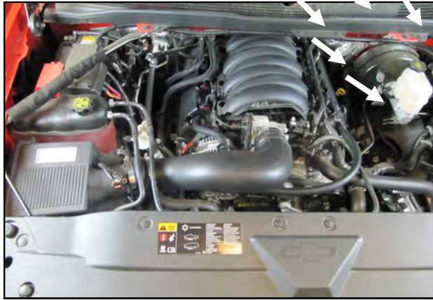
14. Double check your work. Make sure all Clamps are tight and reconnect the negative battery cable.
