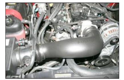
**9.** Install the **MIT** onto the **MAF** first, and then onto the throttle body. Adjust for fit, and tighten the hose clamps. Next connect the breather hose to the factory breather port on the valve cover. Reinstall the factory hose clamp barb back into the hole in the bottom of the **MIT**. Reinstall the engine cover.
