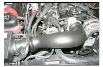
**9.** Install the **MIT** onto the **MAF** first, and then onto the throttle body. Adjust for fit, and tighten the hose clamps. Next connect the breather hose to the factory breather port on the valve cover. Reinstall the factory hose clamp barb back into the hole in the bottom of the **MIT**. Reinstall the engine cover.
