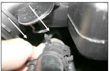
$\bf 3.$  Separate the factory intake tube from the plastic clamp barb that secures the radiator hose to the tube. A firm downward push will usually do it.
