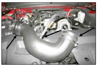
**6.** Install the urethane coupler on the throttle body end of the Modular Intake Tube with two #64 hose clamps. Install the urethane hump hose on the other end of the MIT with the remaining two #64 hose clamps. Leave all clamps loose for now. Install the 3/8" barbed fitting into the MIT, and slide the 3/8" breather hose over the barbed fitting as shown.
