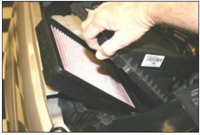
**8.** Install the Airaid Premium filter into the factory airbox, and re-install the 4 screws.
