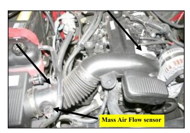
**4.** Loosen two hose clamps on the factory intake tube. One at the throttle body end, and the other at the Mass Air Flow sensor (MAF) end.
