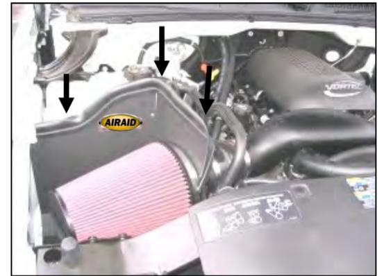
12. Press the weather strip (#8) along the top edges of the Airaid Cool Air Dam; assure that it is fully seated along the edges. (Hint: Begin at a corner and work toward the ends). Mount the Airaid Premium Filter (#1) onto the air filter adapter and tighten the hose clamp.
