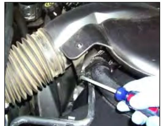
3. Using a flat head screwdriver, gently pry the radiator hose bracket from the factory intake tube assembly and remove the intake tube from the vehicle.
