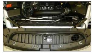
34. Reinstall the upper radiator valence and secure with the ten factory push pins.
