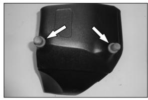
15. Remove both factory air filter housing bushings from the factory housing and install them onto the AIRAID filter housing as shown.
