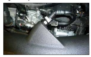
28. Connect the CCV tube to the quick connect fitting installed into the AIRAID intake tube.
