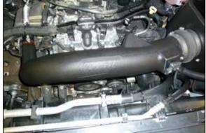
25. Install the intake tube assembly into the coupler at the air filter housing and then into the coupler at the turbo inlet, adjust the tube for best fit and then secure with the provided hose clamps.
