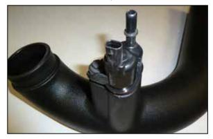
24. Remove the CCV solenoid from the factory intake tube and install it into the K&N intake tube using the factory bolt.
