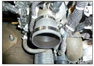
20. Install the provided straight coupler onto the turbo inlet and secure with the provided hose clamp.
