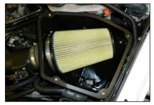
31. Install the AIRAID air filter onto the filter adapter and secure with the provided hose clamp.
