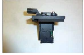
22. Remove the mass air sensor from the factory housing and then install the sensor into the adapter provided along with the gasket.
