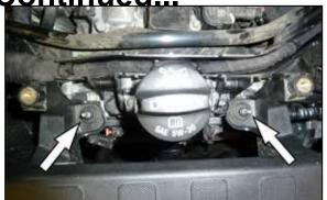
7. Remove the two nuts that secure the intake tube to the engine. Unhook the wiring harness from the intake tube and then remove the intake tube assembly from the vehicle. These nuts will be reused in a later step.
