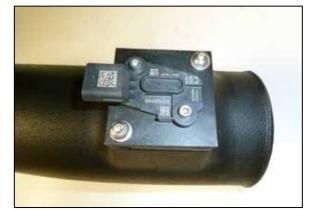
11. Using a small pick or similar tool, release the locking tab that secures the wiring harness bulk connector to the air filter housing and then remove the harness from the housing.
