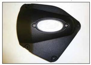
32.Install the AIRAID window into the AIRAID filter housing lid using the provided hardware.
