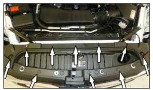
9. Remove the ten push pins that secure the upper radiator valence and then remove the valence from the vehicle.
