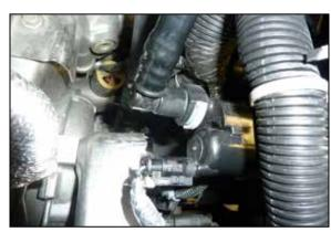
29.Connect the CCV tube to the solenoid and connect the electrical connection.
