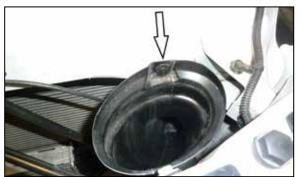
10. Remove the push pin that secures the fresh air duct to the core support and then dislodge the duct from the air filter housing. This push pin will be reused in a later step.
