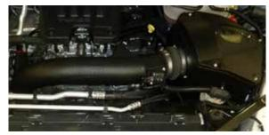
**36. Double check your work!** Make sure there is no foreign material in the intake path. Make sure all clamps, hoses, bolts, and screws are tight. Double check the hood clearance! **Reconnect the negative battery cable!**
