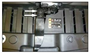
8. Remove the two bolts that secure the hood release latch handle and then remove the handle from the vehicle.
