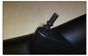
21. Install the provided quick connect fitting into the AIRAID intake tube.
