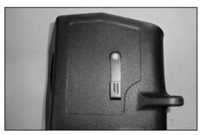
13. Install the provided bulk connector bracket onto the AIRAID air filter housing and secure with the provided hardware.
