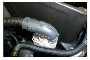
18. Install the wiring harness bulk connector onto the bracket installed onto the AIRAID air filter housing.
