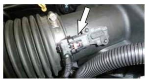
2.Disconnect the mass air sensor electrical connection and loosen the hose clamp that secures the factory intake tube to the air filter housing.
