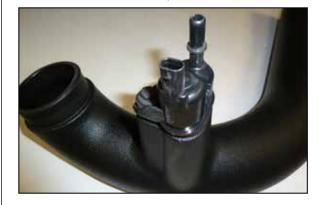
24. Remove the CCV solenoid from the factory intake tube and install it into the K&N intake tube using the factory bolt.
