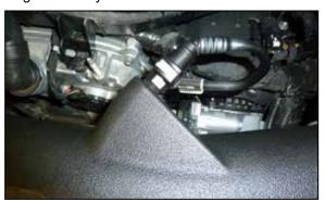
28. Connect the CCV tube to the quick connect fitting installed into the AIRAID intake tube.
