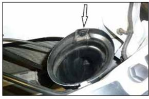
17. Install the fresh air intake duct into the AIRAID air filter housing and then secure it to the core support using the factory push pin.
