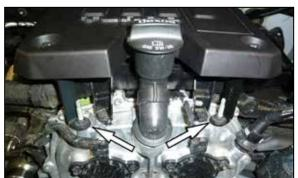
27. Install the engine cover onto the engine and secure the brackets to the factory mounting studs using the factory nuts.
