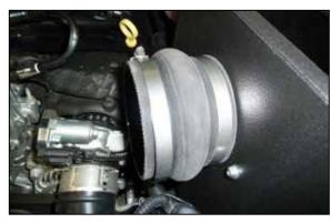
19. Install the hump coupler onto the filter adapter and secure with the provided hose clamp.
