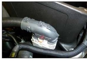
18. Install the wiring harness bulk connector onto the bracket installed onto the AIRAID air filter housing.
