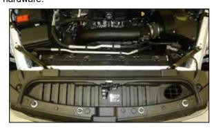
34. Reinstall the upper radiator valence and secure with the ten factory push pins.
