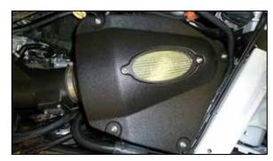
33. Install the AIRAID air filter housing lid onto the lower air filter housing using the provided hardware.
