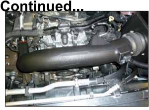
25. Install the intake tube assembly into the coupler at the air filter housing and then into the coupler at the turbo inlet, adjust the tube for best fit and then secure with the provided hose clamps.
