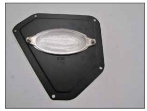
14. Install the AIRAID<sup>®</sup> window into the lid and secure with the provided hardware.
