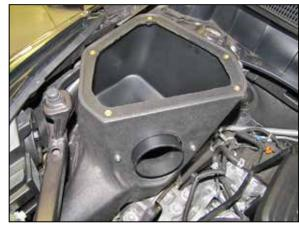
8. Install the AIRAID<sup>®</sup> filter housing into the vehicle.
