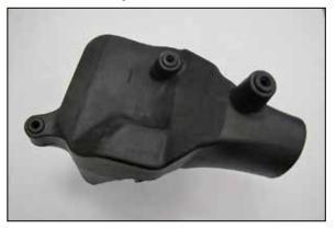
6. Remove the three mounting grommets from the factory air filter housing and install them into the AIRAID<sup>®</sup> air filter housing as shown.
