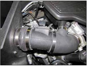
12. Install the AIRAID<sup>®</sup> intake tube assembly into the couplers, adjust the tube for best fit and secure with the provided hose clamps.
