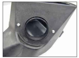
7. Install the filter adapter into the AIRAID<sup>®</sup> air filter housing as shown.
