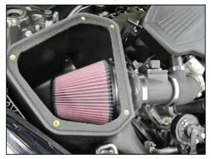
13. Install the air filter onto the filter adapter and secure with the provided hardware.
