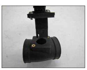
11. Remove the mass air sensor from the factory housing. Install the mass air sensor into the adapter provided and secure with the provided hardware. Install the provided gasket onto the adapter and then install the assembly into the AIRAID<sup>®</sup> intake tube and secure with the provided hardware.
