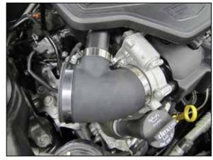
9. Install the provided coupler onto the throttle body and intake plenum. Secure with the provided hose clamps.
