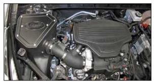
**17. Double check your work!** Make sure there is no foreign material in the intake path. Make sure all clamps, hoses, bolts, and screws are tight. Double check the hood clearance! **Reconnect the negative battery cable!**
