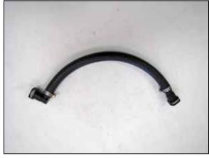
10. Assemble the crank case vent hose assembly as shown.
