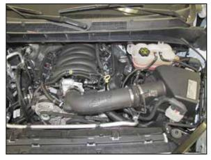
**12. Double check your work!** Make sure there is no foreign material in the intake path. Make sure all clamps, hoses, bolts, and screws are tight. Double check the hood clearance! **Reconnect the negative battery cable!**
