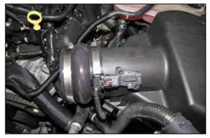
6. Install the provided hump coupler (KITHUMPHS22) onto the air filter and secure with the provided hose clamp.
