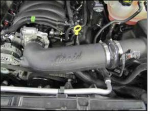
9. Install the AIRAID<sup>®</sup> intake tube into the coupler at the air filter housing and then into coupler on the throttle body, adjust the tube for best fit and then secure with the provided hose clamps.
