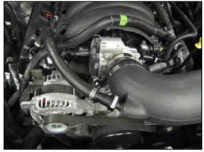
11. Connect the crankcase vent hose assembly to the fitting in the AIRAID<sup>®</sup> intake tube and to the valve cover port.
