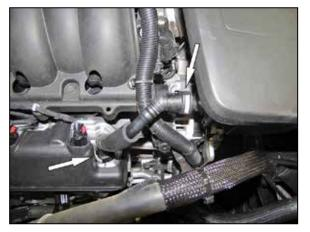
2. Depress the locking tabs and disconnect the crank case vent line from the intake plenum and valve cover.
