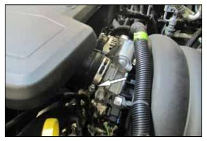
4. Loosen the hose clamp that secures the intake plenum to the throttle body. Rotate the plenum counter clockwise to unlatch it from the mounting bracket and then remove the plenum from the vehicle.
