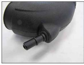
8. Install the provided grommet and vent fitting into the AIRAID<sup>®</sup> intake tube as shown.
