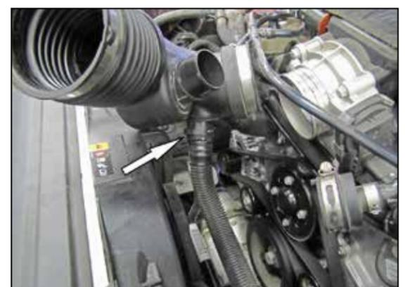
5. Lift up the intake tube to access the sound tube connection and then disconnect the sound tube from the intake tube and remove the intake tube from the vehicle.
