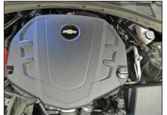
15. Reinstall the engine cover and secure with the factory hardware.
