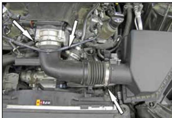
4. Loosen the hose clamp that secures the EVAP line and unclip the crank case vent to the intake tube and disconnect them. Loosen the two hose clamps that secure the intake tube to the air filter housing and throttle body. Disconnect the tube from the air filter housing and throttle body.
