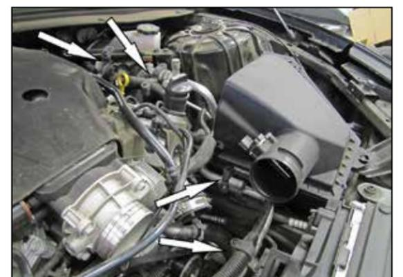
6. Release the four sound drum tube mounts.
