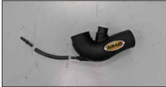
11. Install the provided vent hose and quick disconnect fitting onto the intake tube.
