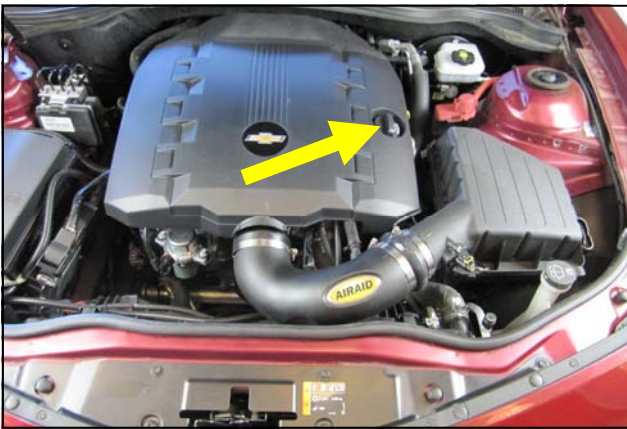
14. Reinstall the engine cover and oil cap. Reconnect the Battery.
