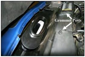
11. Set the Airaid Premium Filter into the area in front of the radiator. It will be mounted in step #
