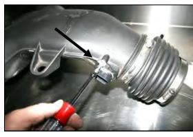
**5.** Using an IPR20 Torx Plus Security Bit (Or Equivalent) remove the two factory screws that hold the **MAF** sensor into the factory intake tube. Remove the **MAF** sensor for reinstallation in step #9.
