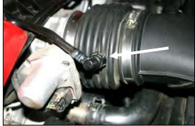
**2.** Push the tab on the top of the crankcase breather connector, and disconnect the breather hose from the factory intake tube breather fitting.
