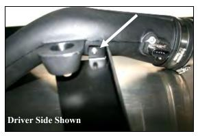
10. Attach the two air dams (#4 driver side & #5 passenger side) onto the Airaid Intake Tube using one 8-32x1/4" button head bolt (#8) and #8 flat washer (#9) on each side. Leave the bolts slightly loose for now to allow for adjustment.
