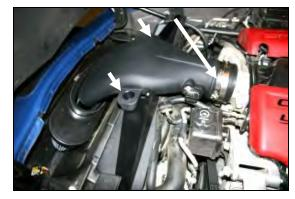
12. Install the Airaid Intake Tube assembly onto the throttle body first, and then align the grommets and the holes in the air dams over the factory grommet posts on top of the radiator shroud. Push down to seat the grommets on the posts. Now tighten the hose clamp on the throttle body.
