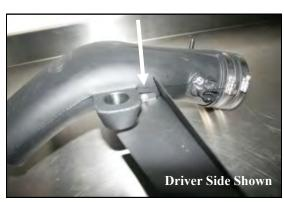
**8.** Attach the two air dams (#5 driver side & #4 passenger side) onto the Airaid Intake Tube using one 8-32x1/4" button head bolt (#8) and #8 flat washer (#9) on each side. Leave the bolts slightly loose for now to allow for adjustment.
