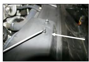
9. Using a flat blade screwdriver, pry up the center pin in the grommet post closest to the right fender on the radiator shroud, and remove both pieces of the grommet post from the vehicle.
