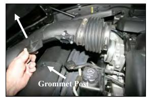
**3.** Lift up on the factory intake tube assembly to disengage the grommets from the three grommet posts and throttle body. Remove the assembly from the vehicle.
