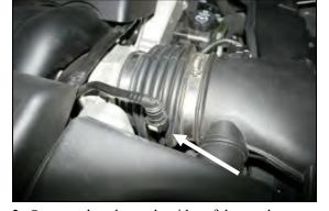
**2.** Squeeze the tabs on the sides of the crankcase breather connector, and disconnect the breather hose from the factory intake tube breather fitting.
