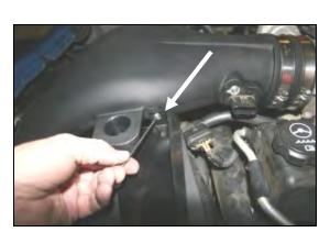
**14.** Tighten all four button head bolts that secure the air dams to the intake tube, and the radiator shroud.
