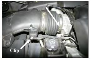
1. **Disconnect negative battery cable.**Remove the grey security clip on the bottom of the Mass Air Flow sensor wiring connector. Next squeeze the tab on the bottom of the connector, and disconnect the wiring harness from the sensor. Now loosen the hose clamp holding the tube to the throttle body.
