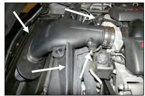
15. Slide the Airaid Premium Filter up onto the end of the intake tube and tighten the clamp. Reconnect the MAF sensor wiring harness and replace the grey security clip. Reconnect the factory breather hose to the breather fitting. Install the weather strip (#6) onto the top of the air dams as
