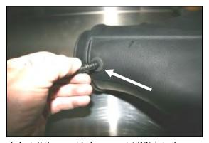
**6.** Install the provided grommet (#13) into the hole in the Airaid Intake Tube (#2). Next install the factory plastic breather fitting removed in step #5 into the grommet.
