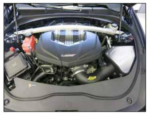
14. Double check your work! Make sure there is no foreign material in the intake path. Make sure all clamps, hoses, bolts, and screws are tight. Double check the hood clearance! Reconnect the negative battery cable!
