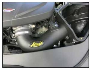
9. Install the intake tube into the air filter housing and then into the coupler on the throttle body, Secure the tube to the filter housing using the provided hardware and then secure the tube to the coupler with the provided hose clamp.
