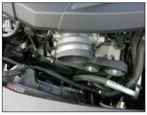
8. Install the provided coupler hose onto the throttle body and secure with the provided hose clamp
