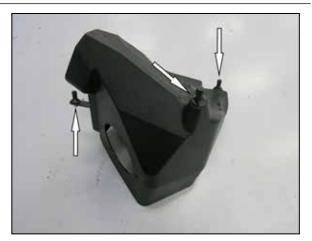
4. Install the provided mounting bracket through the cutline in the AIRAID air box and then secure with the provided hardware. Install the provided mounting studs onto the bracket and onto the air filter housing as shown.
