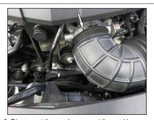
3. Disconnect the crank case vent line and loosen the hose clamp that secures the intake tube to the throttle body. Remove the complete intake system from the vehicle. **NOTE: AIRAID recommends** that customers do not discard the factory intake system.
