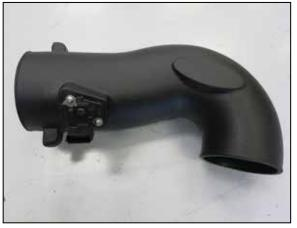
6. Remove the mass air sensor from the factory air filter housing and install it into the AIRAID intake tube using the provided hardware.
