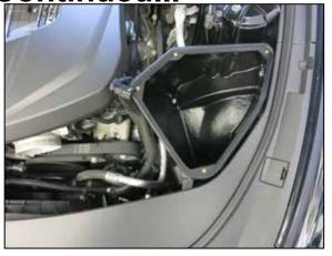
5. Install the AIRAID air filter housing into the vehicle so the mounting studs engage the factory mounting grommets.
