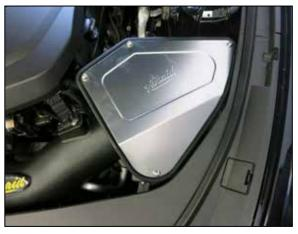
13. Install the provided gasket onto the air filter lid, then install the lid onto the air box and secure with the provided hardware.
