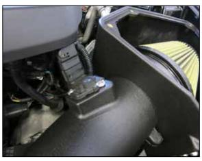
12. Reconnect the mas air sensor electrical connection.
