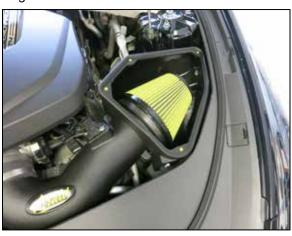
11. Install the AIRAID air filter onto the intake tube and secure with the provided hose clamp.
