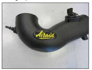
7. Install the provided quick disconnect fitting into the AIRAID intake tube and then apply the provided decal onto the intake tube. NOTE: Plastic NPT fittings are easy to cross thread. Install the vent fitting "hand" tight, then turn it two complete turns with a wrench.
