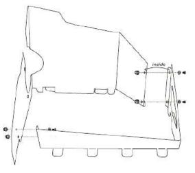
**3.** Assemble Airaid Quick Fit Cool Air Dam panels using the (4) 6/32 screws, washers and nuts provided.
