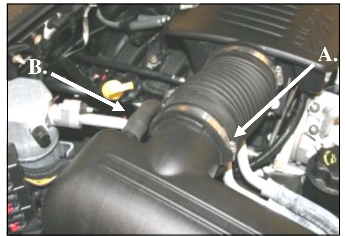
2. A.) Loosen the hose clamp on the factory airbox lid. B.) Disconnect the breather hose from the factory airbox lid.
