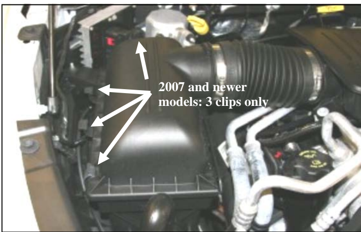
1. Disconnect the negative battery cable. Unlatch the four clips (three on 2007 and newer models) on the factory airbox.
