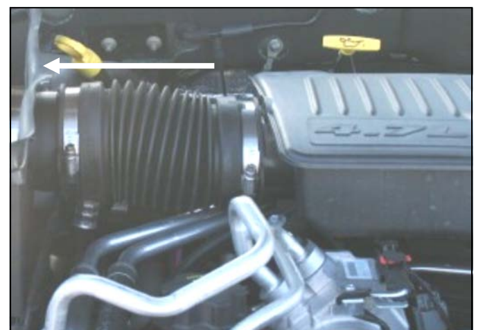
6. Slide the factory intake tube onto the Quick Fit Panel and tighten the hose clamp.
