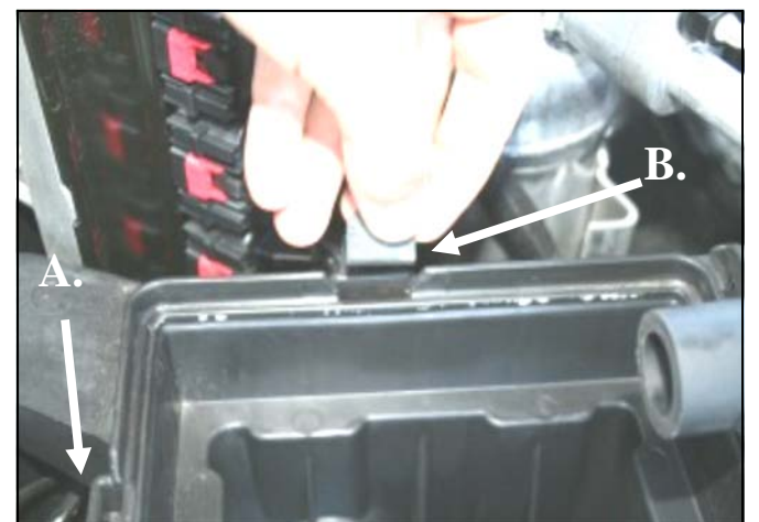
4. 2007 and newer models only: A.) Using a flat blade screwdriver, gently pry and remove one factory clip from the passenger side rear of the airbox base. (see arrow above) B.) Re-install the clip onto the rear of the factory airbox base (see arrow above).
