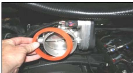
5. Remove the factory seal from the throttle body.
