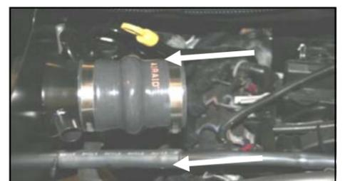
9. Install the urethane hump hose (#4) onto the tube on the Quick Fit Panel using two
