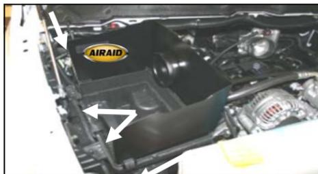
8. Install the Quick Fit Panel (#2) onto the factory airbox base by sliding the tabs on the base thru the Quick Fit Panel and then adjust the sides to fit. Re-latch the 4 clips to hold the Quick Fit Panel securely in place. Apply the Airaid Foil Decal onto the Panel as shown.
