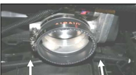
10. Install the reducing coupler (#5), small end first, onto the throttle body using two #52 hose clamps (#8). Leave the clamps loose for now.
