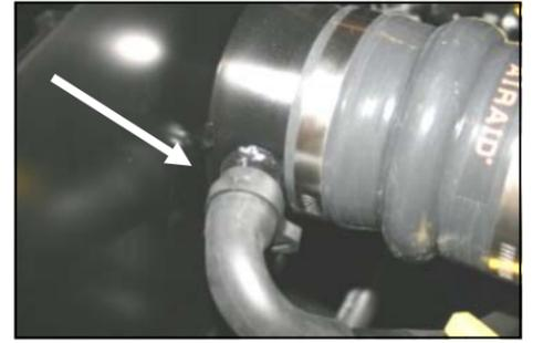
15. Slip the #24 speed clamp (#11) over the factory breather hose and re-connect the factory breather hose to the nipple on the Quick Fit Panel. Squeeze the clamp to retain the hose in place.
