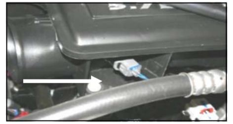
3. Squeeze the tab on the connector, and disconnect the intake temperature sensor.
