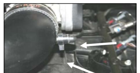
12. Install the provided rubber cap (#7) and speed clamp (#10) onto the nipple on the Modular Intake Tube, as shown.
