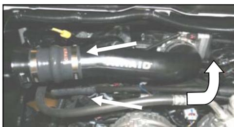
11. Install the Modular Intake Tube (#3) into the hump hose first and then into the reducing coupler. Adjust for fit, and then tighten all 4 hose clamps.
