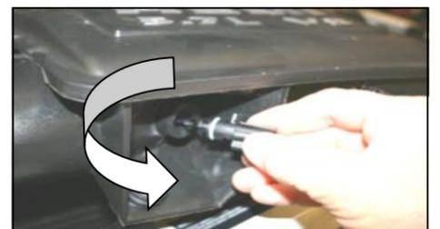
6. Gently twist the air temperature sensor counterclockwise and remove it from the
