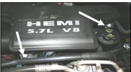
4. Using a 10mm socket, remove two bolts holding the intake resonator to the intake manifold. Lift and pull the resonator away from the
