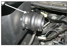
11. Install the hump hose (#4) onto the CAB using two #60 hose clamps (#11). Tighten the hose clamp on the CAB.
