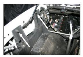
**9.** Remove the two bolts that secure the factory airbox mounting bracket to the inner fender. They will be reinstalled in step #10.
