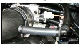
**15. 2002-03 Models:** Install one end of the provided 90° barbed fitting (#22) into the factory breather hose and then connect the supplied 1/2" breather hose (#21) to the other end. Connect the hose to the nipple on the Airaid intake tube. Secure all three connections with the provided #16 Speed Clamps (#17).
