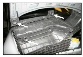
**3.** Turn the factory air box over and remove **3** of the 4 grommets. They will be reinstalled in the Airaid Cool Air Box in step #8.
