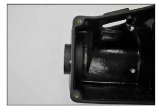
5. Install the filter adapter into the AIRAID® air filter housing and secure with the hardware provided.
