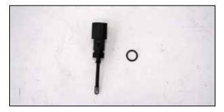
11. Remove the inlet temperature sensor from the factory intake tube and then remove the O-ring from the
