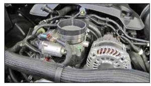
8. Install the provided coupler hose (KITCOUPLER09) onto the throttle body and secure with the provided hose clamp.
