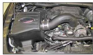
17. Double check your work! Make sure there is no foreign material in the intake path. Make sure all clamps, hoses, bolts, and screws are tight. Double check the hood clearance!
