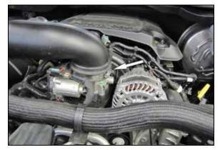
3. Loosen the hose clamp that secures the factory intake tube to the throttle body.
