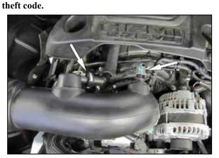
2. Disconnect the inlet air temperature sensor electrical connection and crank case vent quick disconnect fitting.
