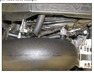
14. Connect the factory crank case vent hose to the quick disconnect fitting installed into the AIRAID® intake tube. Reconnect the inlet air temperature sensor electrical connection.
