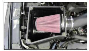
15. Install the AIRAID® air filter onto the filter adapter and secure with the provided hose clamp.
