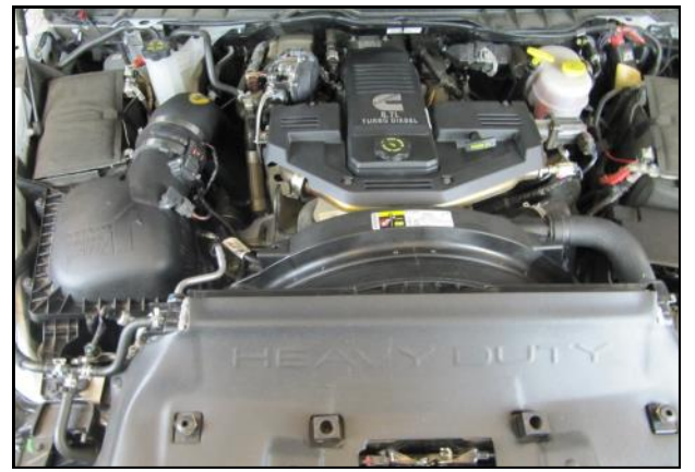
11. Double check your work. Make sure all Clamps are tight and reconnect the negative battery cables.
