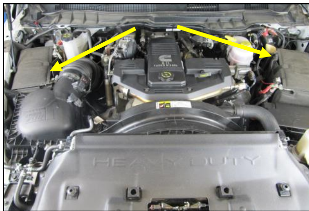
1. Disconnect The Negative Battery Terminals! Warning: Installation of this Intake system requires working in close proximity to the turbocharger. Please allow a sufficient cooling time before beginning the installation to avoid personal injury.
