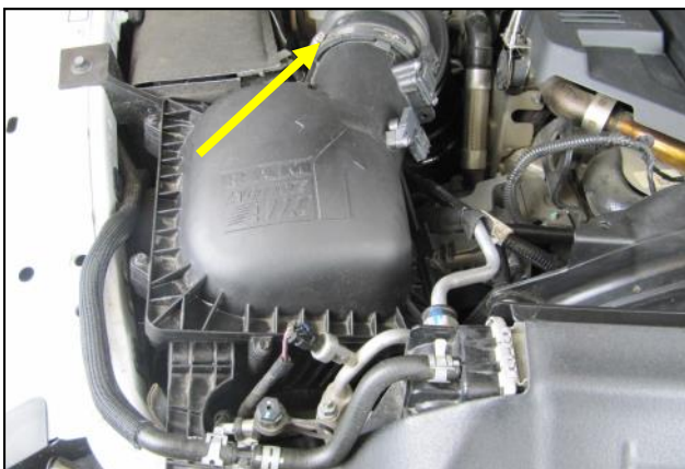
3. Loosen the clamp on the intake tube and remove the airbox lid from the vehicle.
