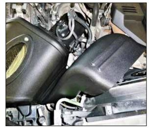
18. Install the AIRAID fresh air intake duct and then install the factory upper portion of the fresh air
