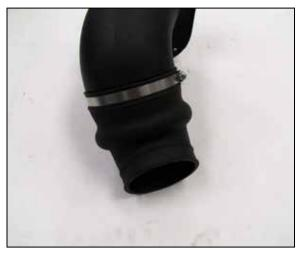
10. Install the flex coupler onto the intake tube and secure with the provided hose clamp. The coupler is keyed and can only be install in one location.
