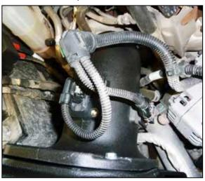
17. Reconnect the air sensor electrical connections.
