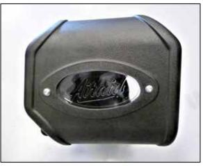
12. Install the AIRAID window into the air filter housing and secure with the provided hardware.
