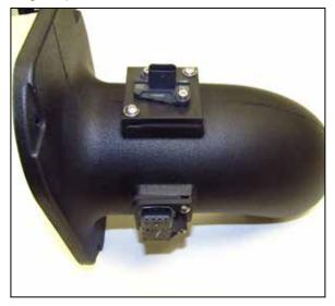
9. Install the two air sensor assemblies into the intake tube using the provided hardware. Be sure the top sensor is installed in the correct direction.
