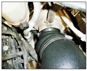
16. Secure the coupler to the turbo inlet with the provided hose clamp.
