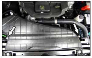
3. Remove the two bolts that secure the fresh air inlet duct to the core support and then remove the inlet from the vehicle.
