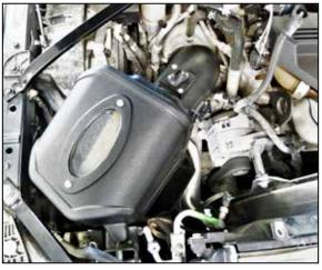
15. Install the intake system into the vehicle so the airbox rests on the mounting studs and connect the coupler to the turbo inlet.
