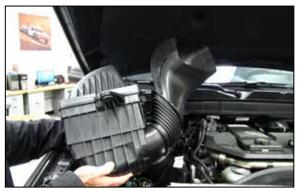
5. Remove the complete air filter housing from the vehicle as shown.
