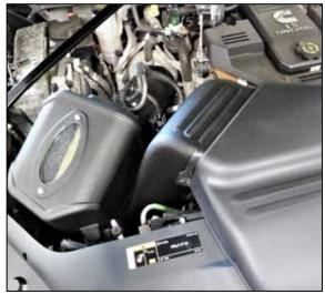
**20. Double check your work!** Make sure there is no foreign material in the intake path. Make sure all clamps, hoses, bolts, and screws are tight. Double check the hood clearance! **Reconnect the negative battery cable!**
