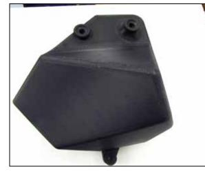
11. Remove the mounting grommets from the factory air filter housing and install them into the AIRAID filter housing as shown.
