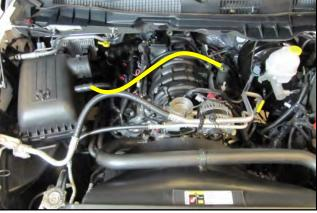
**2.** Remove the PCV line connecting the air box to the valve cover. Note: The 90 degree fitting on the valve cover is to remain in place.
