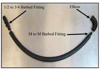
11. Assemble the Airaid PCV line using the 22" breather hose, 1/2" to 3/4" barbed fitting on one end. On the other end, connect the 1/2" elbow to the breather hose using the male to male barbed fitting.
