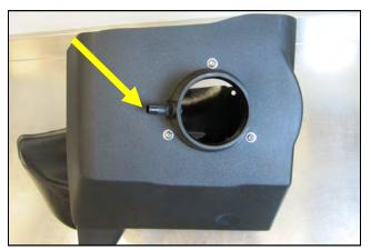
**9.** Install the 1/4" barbed fitting into the cool air box snout as shown.
