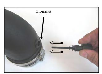
**15.** Insert the 1/2" grommet into the Airaid Intake tube. Transfer the air temperature sensor from the factory intake tube, into the Airaid Tube.
