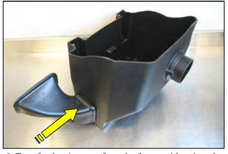
**6.** Transfer the air scoop from the factory airbox into the Airaid cool air box as shown.
