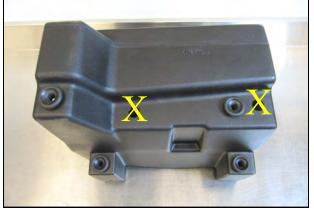
**5.** Transfer the 4 factory air box grommets into the Airaid cool air box as shown. Note: Two of the holes do not receive grommets.
