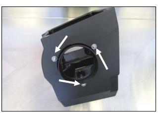
**4.** Install The Filter Adapter in the Cold Air Box using three 1/4- $20 \times 1/2$ " Button Head Bolts and 1/4" Flat Washers.
