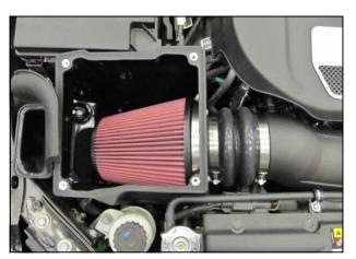
18. Install the Airaid Premium Filter onto the Filter Adapter.
