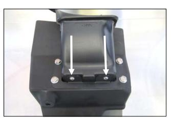
9. Insert the factory air scoop into the Cold Air Box and secure it using two 8-32 x 3/8" Button Head Bolts , #8 Flat Washers, and #8 Kep Nuts.
