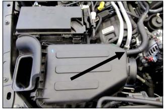
**3.** Disconnect the crankcase breather line in the top of the airbox. Remove the entire airbox as an assembly by unseating it from the mounting grommets in the inner fender and lifting upward.
