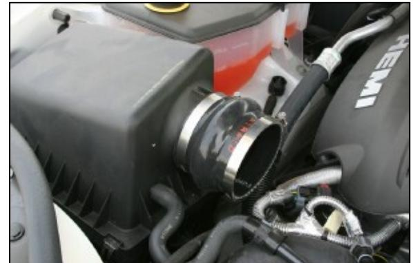
**7. Carefully twist and remove the temperature sensor from the stock intake tube. Remove the stock intake tube from the vehicle.**
