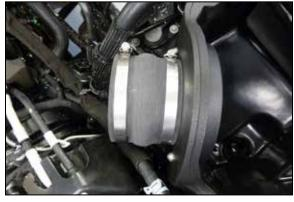
9. Install the provided hump coupler onto the filter adapter and secure with provided hose clamp.
