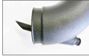
12. Install the provided CCV vent tube into the K&N intake tube as shown. **NOTE: Be sure it is positioned as shown for proper function.**
