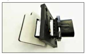
11. Install the mass air sensor gasket onto the sensor adapter. Remove the mass air sensor from the factory housing and install it into the adapter and secure with the provided hardware.
