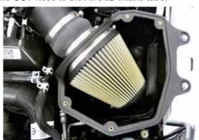
17. Install the AIRAID air filter onto the adapter and secure with the provided hose clamp.
