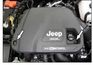
2. Remove the two bolts that secure the engine cover to the engine and then remove the cover from the vehicle.
