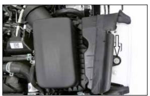
6. Remove the bolt that secures the factory air filter housing to the vehicle and then remove the housing from the vehicle.
