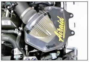
18. Install the Air filter housing lid and secure with the provided hardware.
