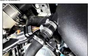
16. Using the provided hose and clamps, connect the CCV hose to the AIRAID intake tube.
