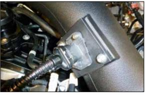
15. Connect the mass air sensor electrical connection.
