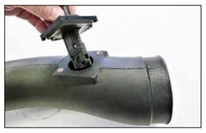
13. Install the mass air sensor assembly into the AIRAID intake tube and secure with the provided hardware.
