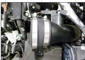
10. Install the provided straight coupler onto the turbo inlet and secure with the provided hose clamp.
