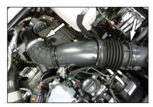
5. Loosen the hose clamp that secures the factory intake hose to the turbo inlet, then release the plastic clamp that secures the hose to the factory air filter housing. Remove the factory intake hose from the vehicle.
