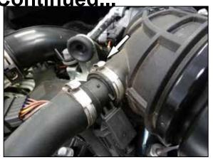
4. Release the one time use clamp that secures the CCV hose to the factory intake hose and then disconnect the CCV hose.
