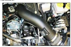
14. Install the AIRAID intake tube into the couplers and adjust for best fit and then secure with the provided hose clamps.
