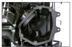
8. Set the AIRAID air filter housing assembly into the vehicle and secure with the provided hardware.
