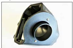
7. Install the filter adapter into the vehicle and secure with the provided hardware.
