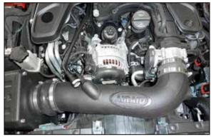
14. Install the intake tube into the hump coupler and then into the coupler at the throttle body, adjust the tube for best fit and secure with the provided hose clamps.
