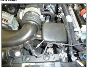
2. Disconnect the inlet air temperature sensor electrical connection and unhook the wiring harness from the intake plenum.
