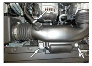
3. Remove the two bolts that secure the intake tube to the core support. Disconnect the crank case vent line, Loosen the two hose clamps and then remove the factory intake tube from the vehicle.
