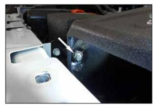
13. Install the air filter housing assembly into the vehicle so the mounting studs insert into the factory air filter housing mounting grommets, then align the housing with rubber mounted stud and secure with the provided hardware.
