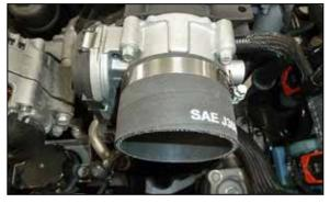
5. Install the provided coupler hose onto the Throttle body and secure with the provided hose clamp.
