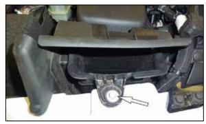
4. Remove the bolt that secures the fresh air duct to the inner fender and remove the factory air box.
