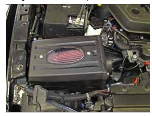
16. Install the air filter housing assembly into the vehicle so mounting studs encage the mounting grommets and then secure the housing to the rubber mounted stud using the provided hardware.
