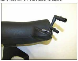
19. Install the O-ring onto the ejector fitting provided and then install the fitting into the AIRAID® intake tube. Secure the fitting with the clip and hardware provided.
