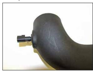
20. Remove the inlet air temperature sensor from the factory intake tube. Remove the O-ring from the sensor and then install into the AIRAID® intake tube using the provided grommet.
