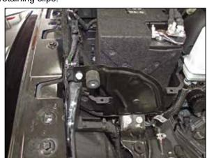
11. Remove the factory bolt and then install rubber mounted stud to replace the factory bolt.
