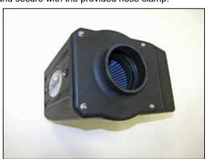
15. Install the air filter assembly into the air filter housing and secure with the provided hardware.
