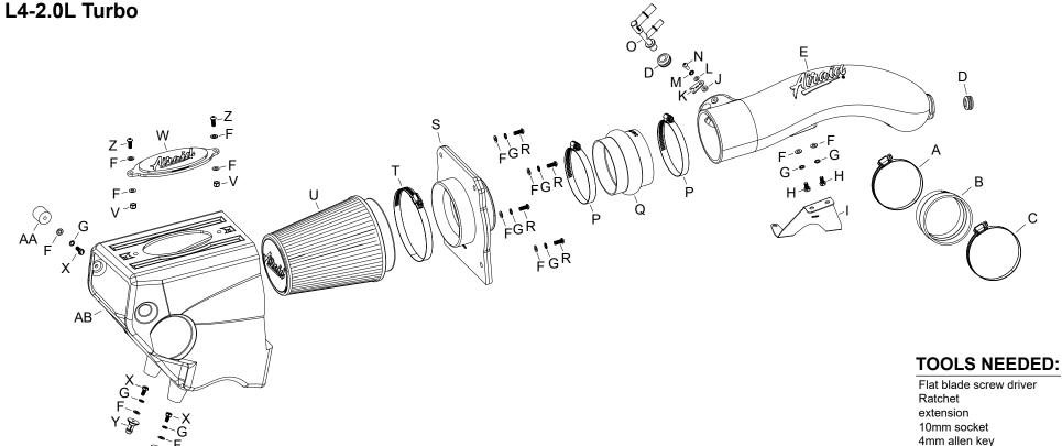
Flat blade screw driver 10mm socket 4mm allen key T20 torx T30 torx
