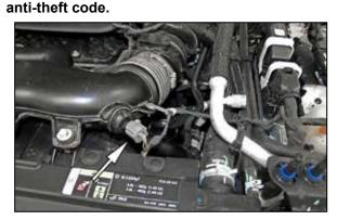
2. Disconnect the inlet air temperature sensor electrical connection and unhook the wiring harness from the intake tube.
