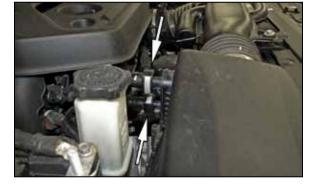
3. Depress the locking tab and disconnect the two vent lines from the air filter housing.
