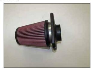
14. Install the AIRAID® air filter mounting adapter and secure with the provided hose clamp.
