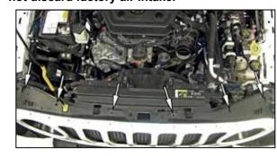
6. Remove the six retaining clips that secure the grill assembly to the core support.
