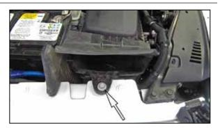
5. Remove the bolt that secures the fresh air duct to the fender. Remove the complete intake system from the vehicle.
