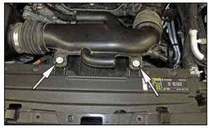
4. Remove the two bolts that secure the intake tube to the core support. Loosen the hose clamp securing the intake tube to the throttle body.
