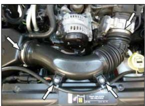
4. Remove the two bolts that secure the intake tube to the core support. Loosen the two hose clamps that secure the intake tube to the throttle body and air filter housing and then remove the intake tube from the vehicle.
