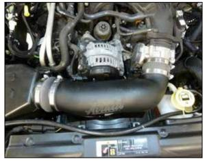
10. Install the AIRAID intake tube into the hump coupler and then into the straight coupler, align for best fit and then secure with the provided hose clamps.
