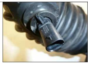
5. Twist the IAT sensor counter clockwise and remove it from the factory intake tube.
