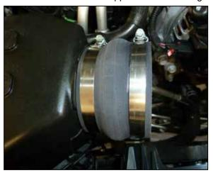
8. Install the provided hump coupler onto the air filter housing and secure with the provided hose clamp.
