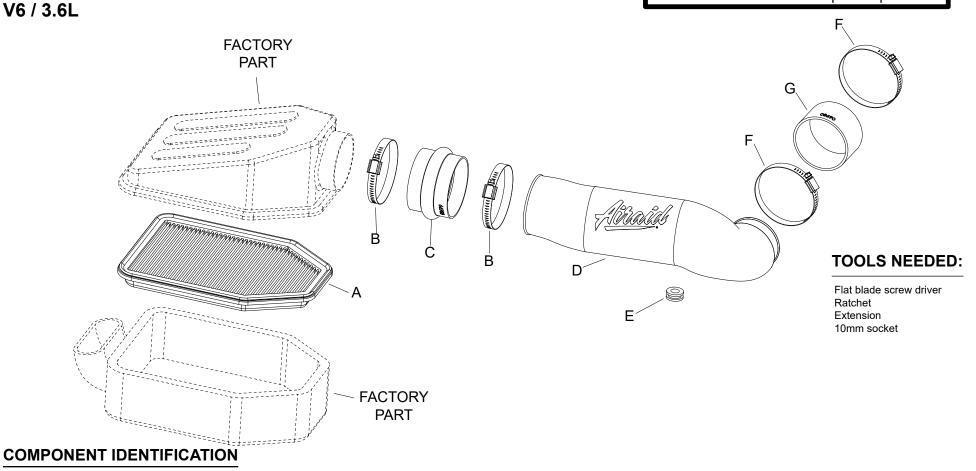
Description Qty. Part # Description Part # Description Part # AIR FILTER HOSE; 3.25"ID X 2"L Α 854-364 D TUBE; AIRAID "OS" 087497 08690 HOSE CLAMP #56 08620 Ε GROMMET; 1/2"ID KITGRMT03 С HOSE; HUMP 3.5"ID X 2.5"L 08699 HOSE CLAMP #52 08610
