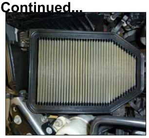
7. Remove the upper air filter housing and then remove the factory air filter. Install the AIRAID air filter and then reinstall the upper air filter housing.
