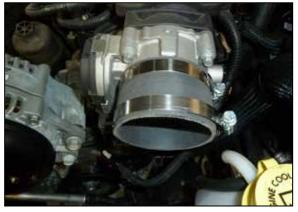
9. Install the provided straight coupler onto the throttle body and secure with the provided hose clamp.
