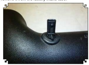
6. Remove the O-ring from the IAT sensor and then install it into the AIRAID intake tube using the provided grommet.
