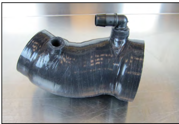
7. Insert the Barbed Elbow Connector into the Airaid Intake Tube as shown.
