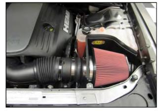
17. Install the Weatherstrip onto the top edge of the Panels with the contour rolling away from the Filter area. Complete the installation by attaching the Airaid Premium Filter to the Filter Adapter.
