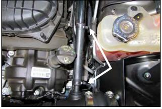
16. For 3.6L V6 Pentastar equipped vehicles: Install the Smaller, 5/8" hose onto the Barbed Fitting and factory hard line. Snap a Speed Clamp on each end of the hose to secure it in place.
