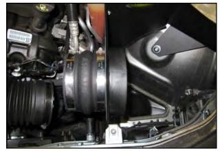
14. Install the Hump Hose and Clamps onto the Filter Adapter. Leave the Clamps loose for now.
