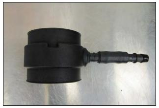
12. For 5.7L V8 HEMI equipped vehicles: Locate the V8 Airaid Intake Tube marked KIT-210-8T and insert the larger, 3/4" Grommet and one of the larger, 3/4" Barbed fittings into the side. Complete the V8 Tube assembly by installing the 2 1/2", 3/4" Hose onto the Tube Fitting, and inserting the second 3/4" Barbed Fitting into it as shown.
