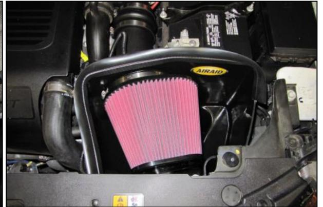
15. Install the Airaid Premium filter onto the Filter Adapter and tighten the clamp. Install the weather strip onto the top of the Air box as shown, with the contour rolling away from the filter.
