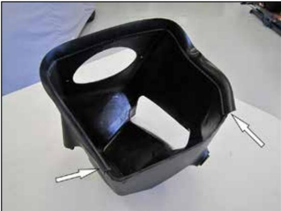
8. Install the provided weather strip onto the AIRAID® housing as shown.
