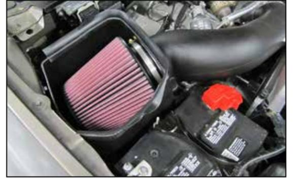
13. Install the air filter onto the intake tube and secure with the provided hose clamp.
