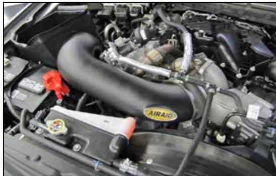
12. Install the AIRAID® intake tube into the AIRAID® housing and into the coupler at the turbo inlet. Adjust the tube for best fit and then secure with the provided hardware and hose clamp.
