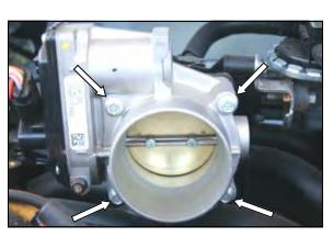
2. Remove the four bolts (and/or nut and stud) from the throttle body, and remove the throttle body from the intake manifold, and set it aside. Retain the wiring harness anchor from the upper left stud on the Explorer for reinstallation in step #4.
