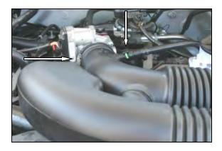
**5.** Re-install the factory intake tube onto the throttle body and tighten the hose clamp. Re-connect the breather hose to the factory intake tube. **Re-connect the negative battery cable!**
