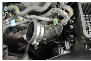
7. Install the provided coupler hose (5-400) onto the driver's side turbo inlet tube and secure with the provided hose clamp.
