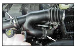
5. Loosen the two remaining hose clamps that secure the factory intake tube to the turbo inlet tubes and then remove the intake tube from the vehicle.
