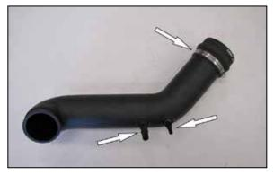
6. Install the provided vent fittings into the AIRAID® intake tube as shown. Install the provided hump coupler (08683) onto the intake tube and secure with the provided hose clamp.
