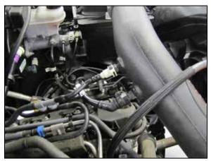
9. Connect the EVAP and crank case vent lines to the quick connect fittings installed into the AIRAID® intake tube.
