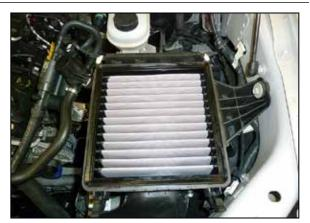
5. Install the provided AIRAID® air filter and reinstall the factory upper air filter housing.
