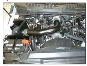
**23. Double check your work!** Make sure there is no foreign material in the intake path. Make sure all clamps, hoses, bolts, and screws are tight. Double check the hood clearance!
