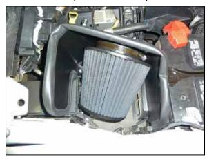
14. Install the heat shield assembly into the vehicle so that the mounting studs insert into the factory air filter housing grommet locations.
