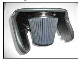
13. Install the AIRAID air filter onto the filter adapter and secure with the provided hose clamp.
