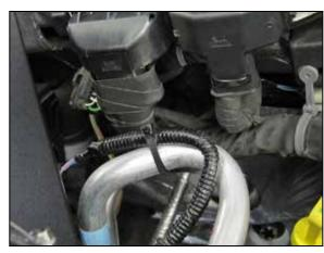
17. Secure the wiring pigtail from step #5 to the A/C line with the provided tie wrap.
