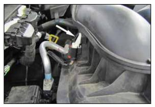
5. Unhook the wiring pigtail from the upper air filter housing.
