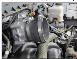
16. Install the provided step coupler (08497) onto the throttle body and secure with the provided hose clamp.
