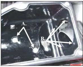
**12.** *A.)* Insert two billet rivet/box mounts (#10) through the bottom of the Airaid Cool Air Box and into the factory grommets. *B.)* Using four stainless steel ½-20x1/2" button head bolts (#6) and 1/4" flat washers (#7), mount the Airaid Intake Tube to the airbox
