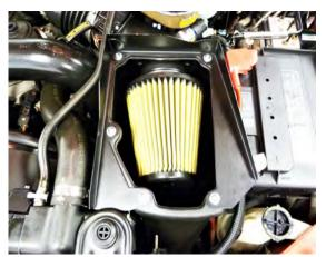
**16.** Install the Top Panel (#4) onto the top of the Airaid Cool Air Box using five stainless steel  $\frac{1}{4}$ -20x1/2" button head bolts (#6) and 1/4" flat washers (#7).
