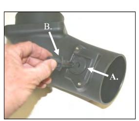
**8.** *A.)* If you have the temperature sensor shown in step #5, install the supplied grommet (#9) as shown above. *B.)* Install the factory air temperature sensor as shown and then the factory grommet and filter restriction gauge. Skip to step #10.
