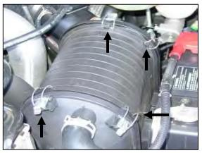
1. <u>Disconnect the negative battery cables.</u> Unlatch all four clips on the factory airbox.
