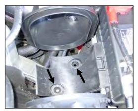
**3.** The factory airbox is held in place by two rubber grommets. Pull straight up and remove the box. (*Note: make sure the factory grommets remain in the lower airbox support.*)
