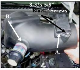
**9.** *A.)* If you have the **MAF** sensor shown in step # 6, install the gasket (#12) and sensor using two *(black)* 8-32x5/8" button head bolts (#11). *B.)* Install the factory grommet and filter restriction gauge.
