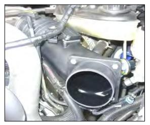
10. Slide the Airaid Intake Tube (#3) into the factory flexible turbo inlet hose. (Note: Do not tighten the hose clamp until assembly is complete.) Reconnect the sensor wiring harness (to the temperature sensor, or the MAF sensor, whichever is present on your vehicle.)
