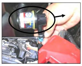
4. Disconnect the electronic filter restriction gauge wiring harness, remove the restriction gauge, and the rubber grommet. (Note: retain these parts for reuse.) Remove the air filter inlet tube and hose assembly (see inset picture). USE CAUTION when removing these elements, as it is a tight fit. Be careful not to tear the factory insulation around the radiator support.
