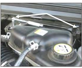
**14.** Factory tolerances may vary between the **MAF** sensor and the coolant reservoir. Therefore, *it may be necessary* to loosen the two 5/16" mounting bolts and adjust the reservoir for better clearance.
