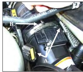
**6. IF YOU HAVE A MASS AIR FLOW SENSOR LIKE THIS,** *A.) D* isconnect the **MAF** sensor wiring harness, remove the two screws using the provided T-20 security bit, and remove the sensor. (*Note: retain the sensor for reuse.*) *B.*) Using a 5/16" socket, loosen the hose clamp on the end of the intake tube.
