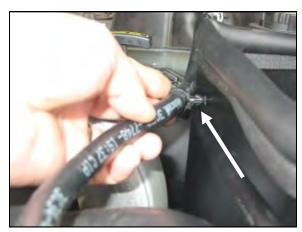
**18.** Spread the black hose mount (#8) over the radiator overflow hose and insert the tab through the hole in the side of the top panel.
