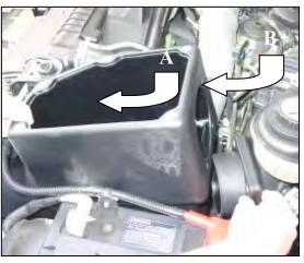
**11.** *A.)* Install the Airaid Cool Air Box (#2) by inserting the long extension of the box into the radiator support. (Note: Make sure the cool air box inlet is not blocked by the factory insulation.) *B.)* Insert the Airaid Intake Tube into the airbox hole.
