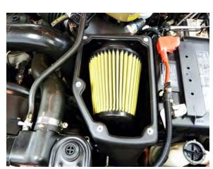
**15.** Install the Airaid Premium Filter (#1) onto the Airaid Intake Tube inside of the airbox, and tighten the hose clamp.
