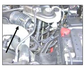
7. Remove the factory intake tube assembly. (Note: do not remove the factory flexible turbo inlet hose from the turbo housing.)
