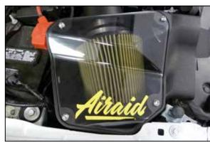
16. Install the AIRAID cover onto the air filter housing and secure with the provided hardware.
