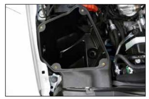
8. Install the AIRAID filter housing and secure with the factory bolt removed in step #6.
