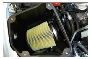
11. Set the AIRAID air filter Into the filter housing.
