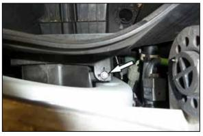
6. Remove the bolt securing the air filter housing and then remove the housing from the vehicle.
