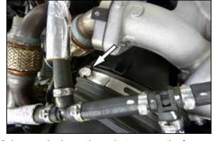
3. Loosen the hose clamp that secures the factory intake tube to the turbo inlet pipe.
