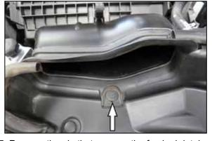
5. Remove the pin that secures the fresh air intake duct.
