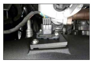
15. Reconnect the mass air sensor electrical connection.
