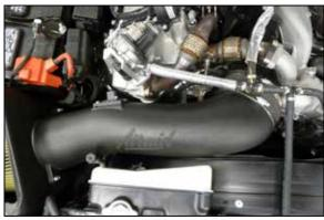
13. Install the intake tube assembly into the air filter housing and secure with the hardware provided. Align the coupler with the turbo inlet and secure with the provided hose clamps.
