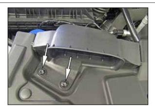
3. Remove the two bolts that secure the factory fresh air intake duct and then remove the duct from the vehicle.
