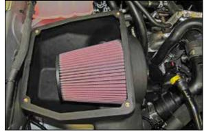
11. Install the air filter assembly into the housing and secure with the provided hardware.
