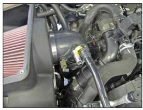
13. Install the coupler onto the intake plenum and connect to the filter adapter, adjust for best fit and secure with the provided hose clamps.
