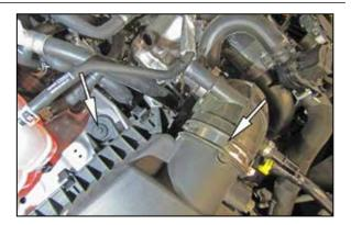
5. Remove the rear air filter housing mounting bolt and loosen the hose clamp that secures the intake hose to the housing.
