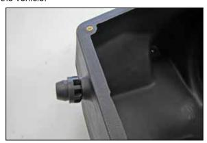
8. Remove the factory air filter housing mounting post and install it onto the AIRAID® air filter housing as shown.
