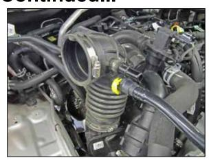
7. Loosen the hose clamp that secures the intake hose to the plenum and then remove the hose from the vehicle.
