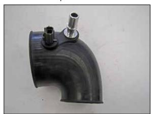
12. Remove the inlet air temperature sensor from the factory housing and remove the O-Ring from the sensor, Install the sensor into the AIRAID® coupler. Install the provided quick disconnect fitting into the AIRAID® coupler as shown.
