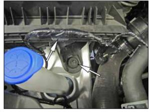
4. Remove the front air filter housing mounting bolt and unhook the wiring harness from the housing.
