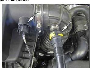
2. Disconnect the inlet air temperature sensor electrical connection and disconnect the crank case vent line from the factory intake tube.
