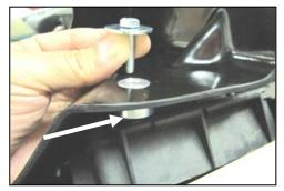
Install the air filter adapter (#6) into the 7. Cool Air Dam (#7) as shown, using 3 button head bolts (#9) and 1/4" flat washers (#10).
