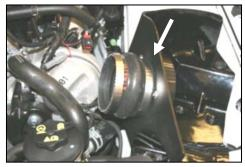
**10.** Install the hump hose (#5) on the filter adapter (#6), with two #72 hose clamps (#13). Tighten only the clamp next to the CAD.
