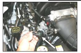
Disconnect negative battery cable. 1. PLEASE READ #22 ON THE BACK PAGE!! Push the green plastic tabs, and remove breather hose from vehicle. (Save for later use).
