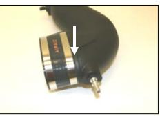
**14.** Install the oval coupler (#4) with two #72 hose clamps (#13). Tighten <u>only</u> the clamp closest to the aluminum fitting. (*Hint: For a clean look, locate the hose clamp tightening screws under the tube)!*
