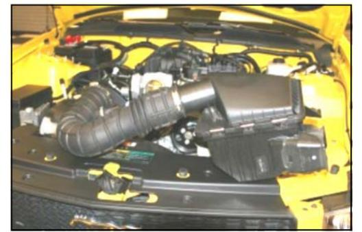
3. Remove the complete intake system as an assembly.
