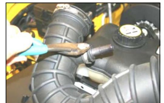
6. With a pair of side cutters, remove the metal band that holds the plastic breather fitting in the factory tube. Next remove the fitting from the tube, and save it for reinstallation in step #11.
