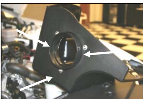
7. Install the air filter adapter (#5) into the Cool Air Dam (#6) as shown, using 3 button head bolts (#8) and 1/4" flat washers (#9).
