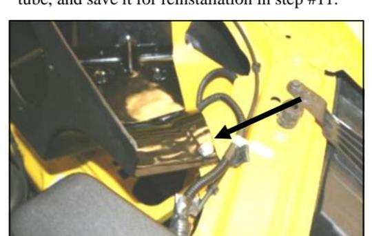
9. If your vehicle has the optional anti-lock brakes, remove the bolt from the bracket under the CAD, and reinstall it thru the hole in the front of the CAD. (See arrow). If your vehicle does not have this bracket, install the supplied 1/4" bolt (#14), two 1/4" washers (#9), and 1/4" Nylock nut (#15) thru the CAD and sheet metal, and tighten.
