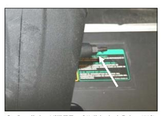
**8.** Install the 1/8"NPT x 3/16" barbed fitting (#13) into the small threaded hole in the side of the Airaid Intake Tube.
