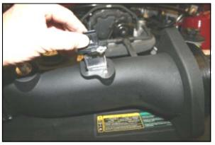
9. Install the Mass Air Flow sensor removed in step #5, into the Airaid Intake Tube using the provided 8-32 x 3/8" button head screws (#8). Make sure the arrow on the sensor is pointing towards the throttle-body.
